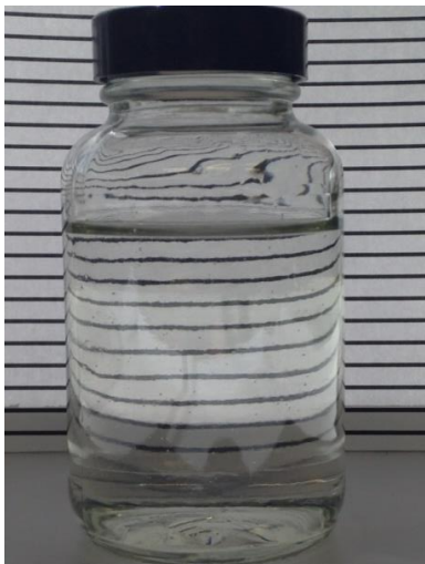
HYPERLAST™ LU 153 FC Polyol Colourless, clear liquid at 40°C
